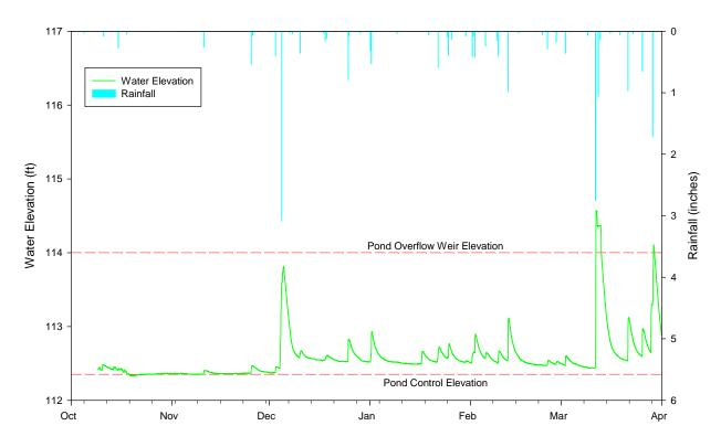
Figure 3-6. Water Surface Elevations in the Pioneer Key Pond from October 2009-March 2010.
