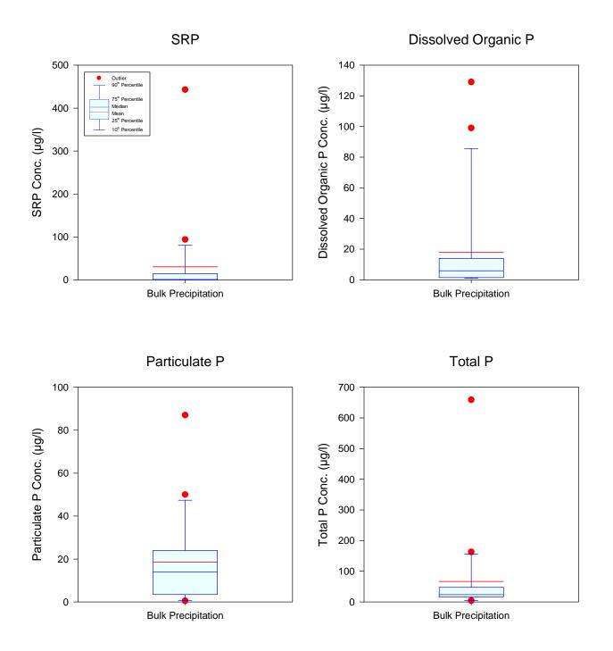
Figure 3-15. Summary of Statistical Variability in Phosphorus Species Measured in Bulk Precipitation Samples at the Pioneer Key Detention Pond Site.
