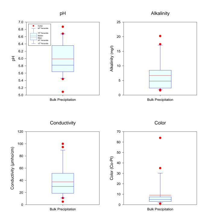
Figure 3-13. Summary of Statistical Variability in General Parameters Measured in Bulk Precipitation Samples at the Pioneer Key Detention Pond Site.
